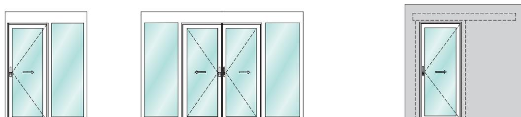
Example of Janisol 2 EI30 fire-resistant sliding door without emergency exit function
