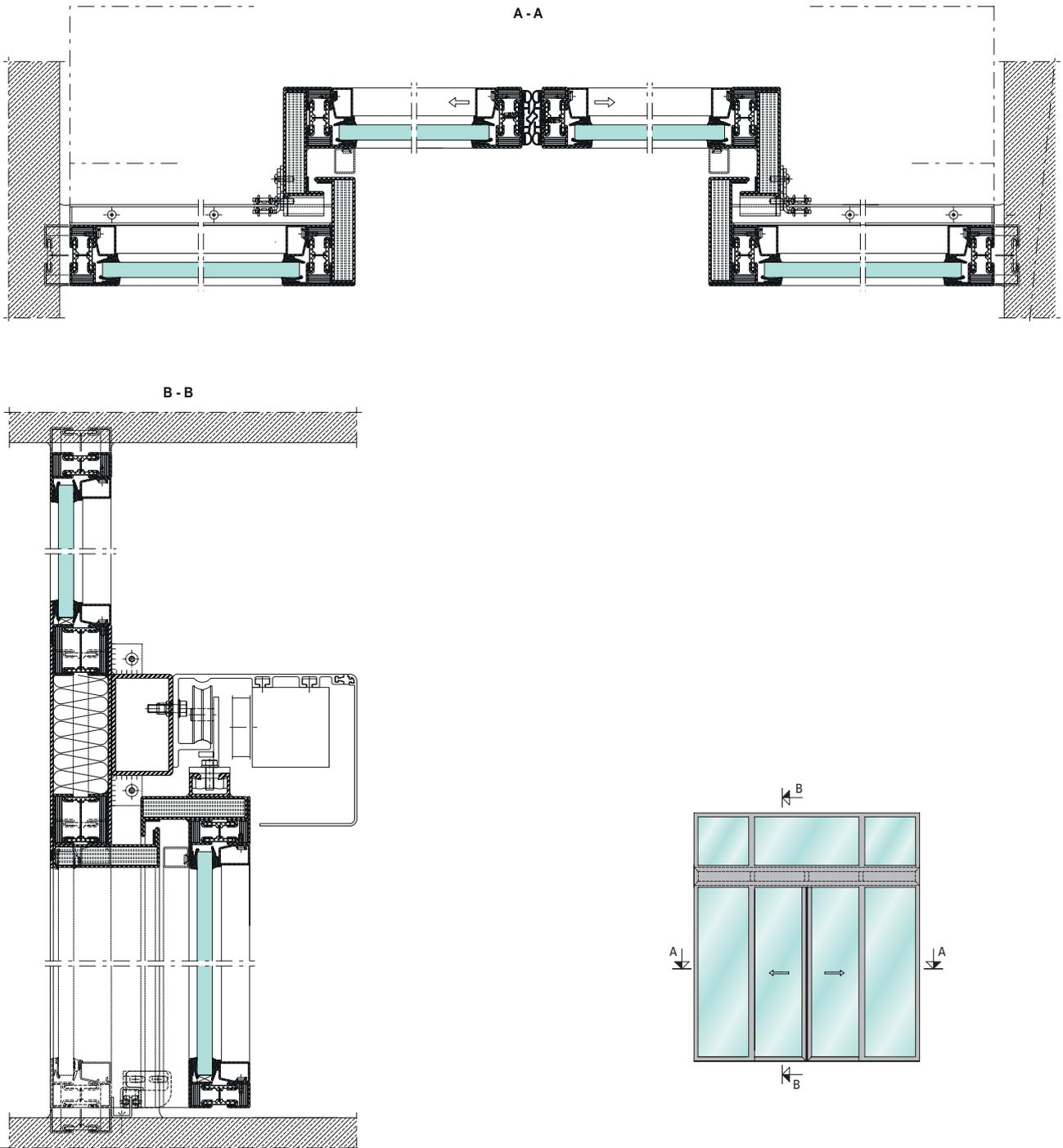
Example of Janisol 2 EI30 fire-resistant sliding door with break-out emergency exit function
